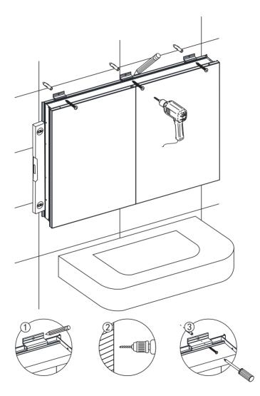
Install glass shelf board and cover plate according to diagram.
