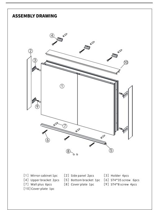
Mark holes based on the desired location, then drill holes and fix mounting bar on the wall
