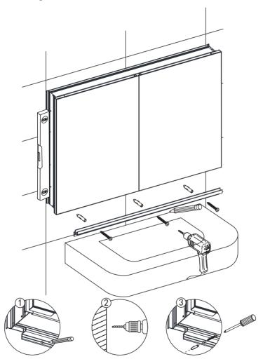
Install the holder,then install side panel.
